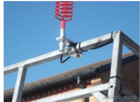
*The same roofrack mounting from further away - notice it's fixed to the top bar of the rack, getting the aerial away from any metal around it*
