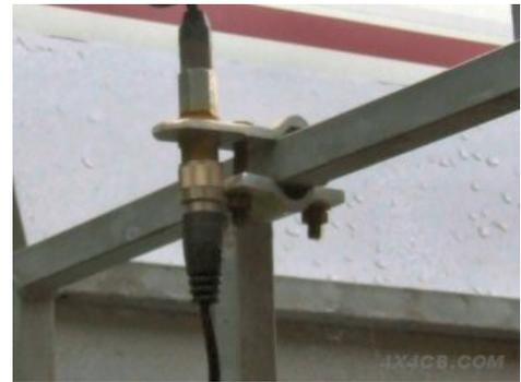
*A two-bolt mount fitted to a galvanised roofrack on a Land Rover*
