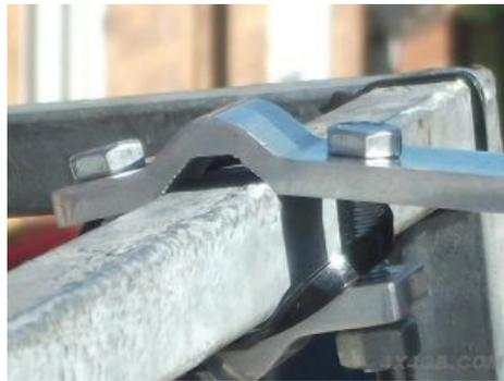
*A close-up of a 2-Bolt bar mount on a roofrack - you can just make out where the galvanised layer has been scraped off to get an earth connection*
