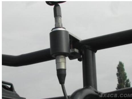
*2-Bolt mount fitted with an [Artificial Ground Plane](#) fixed to a powder coated roofrack that the customer didn't want to scrape in order to get an earth connection*
