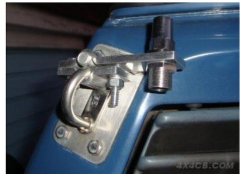
*A 2-Bolt bar mount fitted to an awning tie on a VW Camper*
