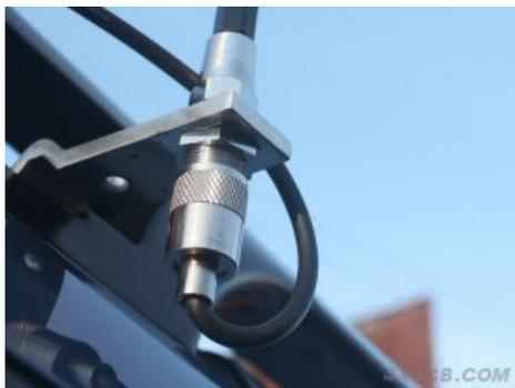
*Here the customer discarded one part of the mount and just bolted the rest to the vehicle using the bolt that holds the roof bars on*
