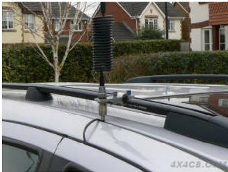
*A two bolt bar mount mounted on the roofbars of an estate car*
