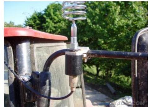
*Another 2-Bolt mount fitted with artificial ground, on the mirror arm of a tractor which does not have a continuous metal-to-metal contact with the rest of the cab*
