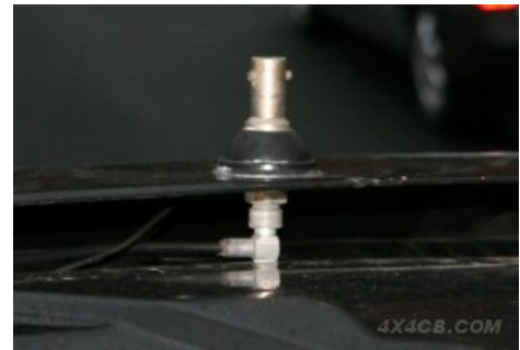
Here's a dome mount (with part of a quick release adaptor fitted) fixed to a rear spoiler on a car - the spoiler isn't metal so an earth lead has been fitted to go to a suitable earthing point
