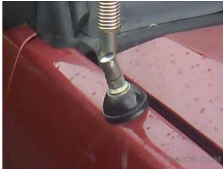
Wing mounting, using our Angle Adaptor to get the aerial vertical
