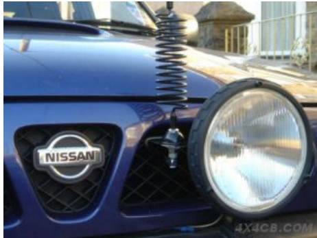
A great idea - a customers homemade bracket for fixing an aerial to the front of his Nissan Terrano
