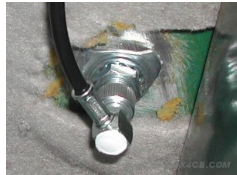
This customer didn't want to go through the business of dropping his headlining to install a dome mount so he just cut a bit out!
