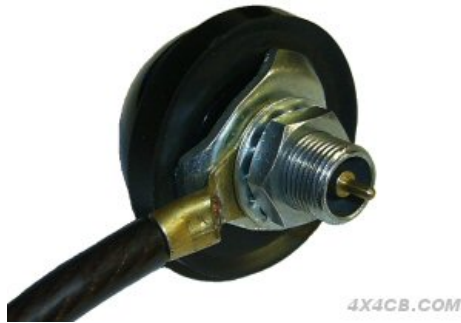
Dome mount with an earthing wire fitted - ring terminal between the washers, with 8awg cable
