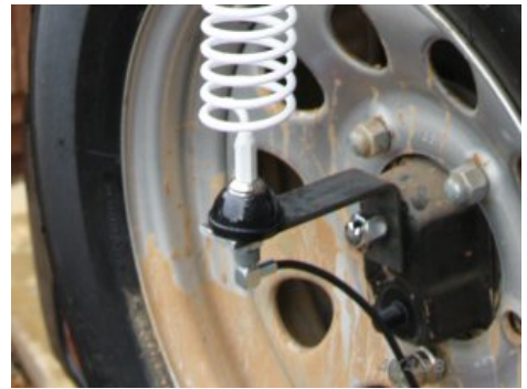
Dome mount on a homemade bracket that the customer fixed to his spare wheel carrier
