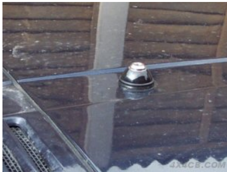
Dome mount fitted to the bonnet of a Jeep
