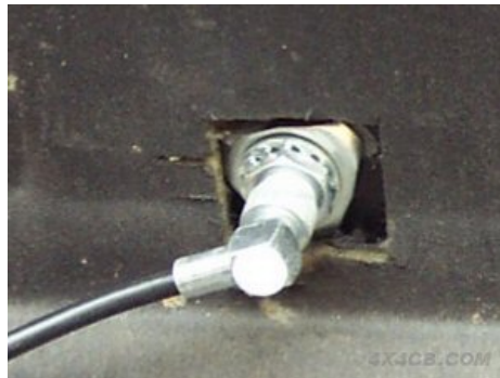
This is a dome mount mounted on a bonnet - the sound deadening material under the bonnet has been cut away to allow the paint to be scraped away and the mount fitted in place
