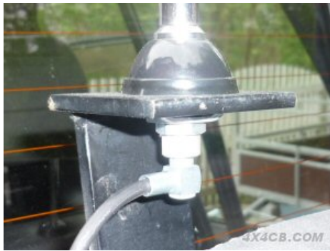
Dome mount fitted to one of those "up and over" wheelcarrier mounts that some chap makes up and sells on Ebay
