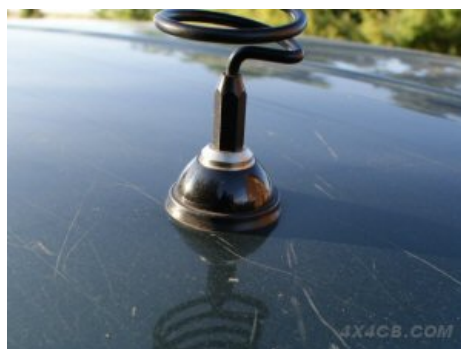
Dome mount through the roof - almost always the best way of mounting a CB aerial (if you don't mind drilling your roof)
