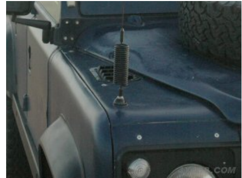
Here's a dome mount on the front wing of a Land Rover defender
