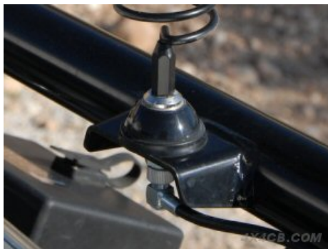
Dome mount fitted to the factory fitted aerial bracket on an ARB bullbar
