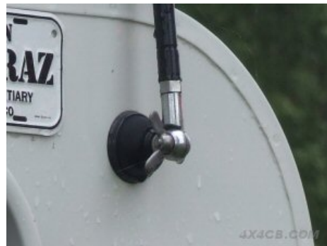
Dome RM fitted to the rear of a Land Rover Defender
