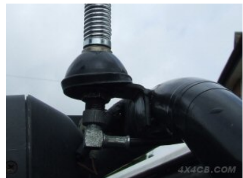
Dome mount fitted to a homemade bracket that the customer had welded to his rollcage
