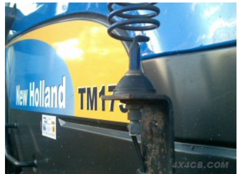
Here a farmer customer made a long bracket to bring the mount up to a suitable height
