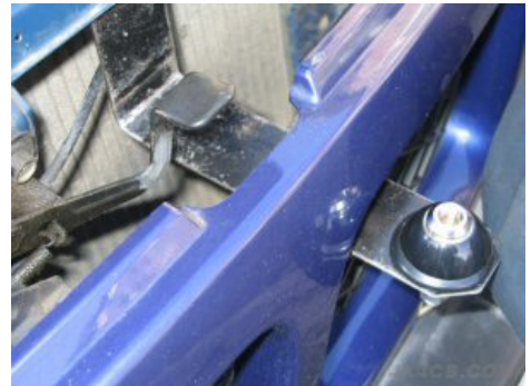
Here's how the Terrano bracket fixes... easily adaptable for other vehicles
