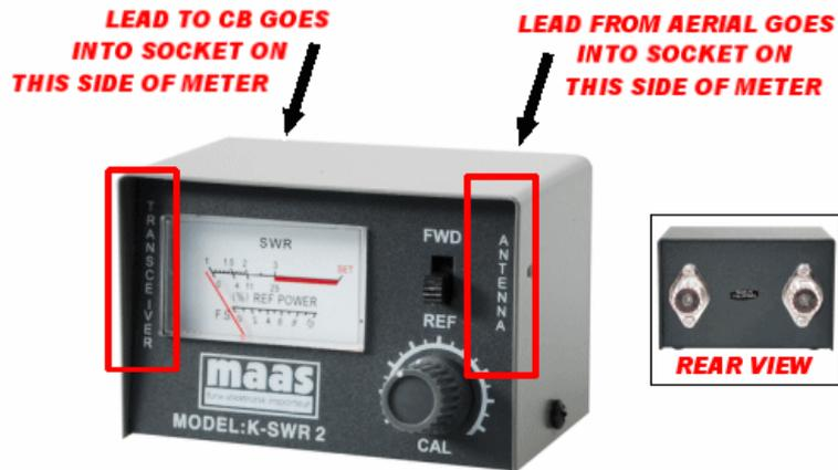
On the meter you will have a calibration control knob, and a switch with two settings. One may be marked FWD, DIR, or CAL and the other marked REF. These stand for forward power (to the aerial) and reflected power (back from the aerial).
